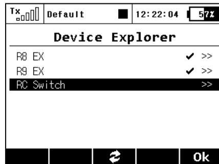
displayed or only displayed as a device ID. The check mark tells you that the device is ready and that you can configure it. By using **F(3)** “Refresh” button you can reset the displayed devices, forcing the auto-detection to explore all attached devices. Otherwise, the process of detecting remote sensors is always running in the background.
